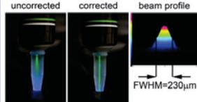
**Fig. 1.** Preconditioning of the 473-nm laser beam and the beam profile.
