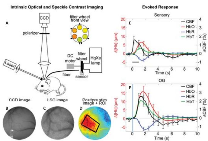
**Fig. 3. IOI and SC.** A) Custom-built combined imaging system [2]. B) CCD image of cortex through a cortical window showing optical fiber used for OG stimulation at the surface. C) Speckle contrast image of the same window as in B. D) Ratio of post- (1-3 s) to pre- (-2.0 s) stimulus [HbO] map showing the region of activation and ROI used for timecourse extraction. E-F) Group- and ROI-averaged timecourses for sensory (E; N = 11) and OG (F; N = 3) stimulation.
