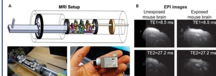
**Fig. 5. BOLD MRI imaging in awake mice.** A) Custom-built MRI-compatible mouse holder with real-time monitoring, stimulus and reward delivery. B) Dual-echo EPI images of a mouse with (right) and without (left) chronic cortical exposure. The cranial window creates susceptibility artifacts.
