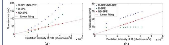
Fig. 4. Dependence of fluorescence intensity on power of NIR and IR [3]. (a) Dependence on NIR power (IR power is fixed at  $4.16 \times 10^{23}$  photons/cm<sup>2</sup>s). (b) Dependence on IR power (NIR power is fixed at  $1.18 \times 10^{23}$  photons/cm<sup>2</sup>s).
