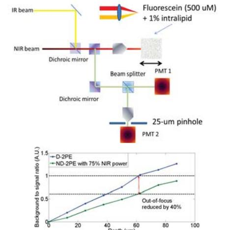
Fig. 9. Excitation with spatially displaced NIR and IR beams. Top: experimental setup. Bottom: signal to background ratio at different depths in scattering medium.
