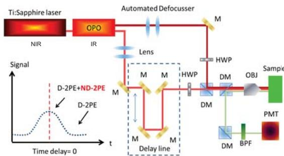
Fig. 2. Experimental setup for demonstration of ND-2PE. HWP, half wave plate; DM, dichroic mirror; OBJ, microscope objective; BPF, band pass filter; PMT, photomultiplier. M, mirror.
