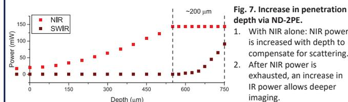
Fig. 7. Increase in penetration depth via ND-2PE.
