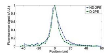
Fig. 8. Axial resolution with 0.55-NA objective lens.
