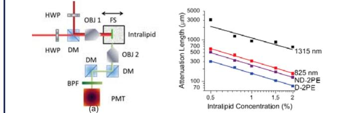
Fig. 5. Attenuation in scattering medium. (a) Experimental setup. (b) Attenuation length as a function of intralipid concentration.
